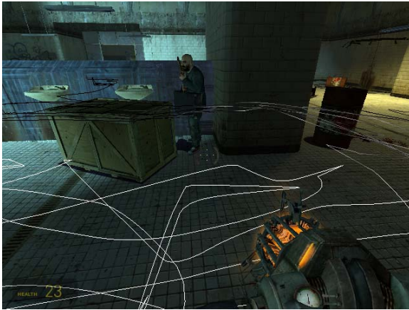
Figure 3. A Half-Life screenshot demonstrating the effects of absorption of photons by different materials. On the left side a wooden box blocks the source from the detector, on the right side a thick concrete wall, and in the back a lead wall. The effects of absorption due to different materials are demonstrated by the difference in intensities received behind different materials.
