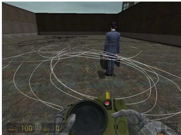
Figure 1. A Half-Life 2 screenshot demonstrating the probability of receiving radiation decaying over distance. The detector traces of shades white to black correspond to high to low probability of receiving radiation at that segment by the detector.
