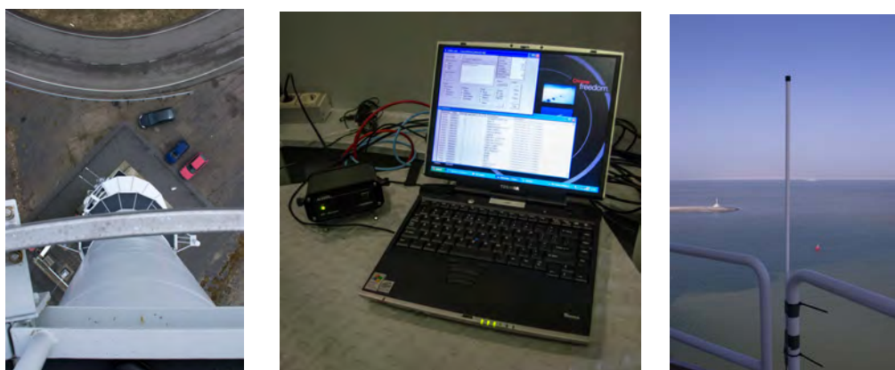
Figure 5. A high tower, laptop to log data and VHF antenna
